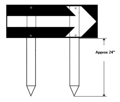
A Direction Marker consists of a 10mm thick Board 4 feet by  $1\frac{1}{2}$  feet with a PVC printed fluorescent yellow arrow on a black background with 2 wooden legs/uprights measuring 2 inches x  $1\frac{1}{2}$  inches x 42 inches as attachments.
